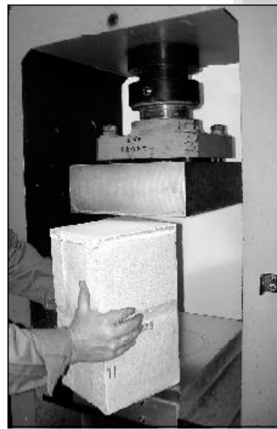
Figure C 1314-11: Positioning Specimen in Compression Machine
